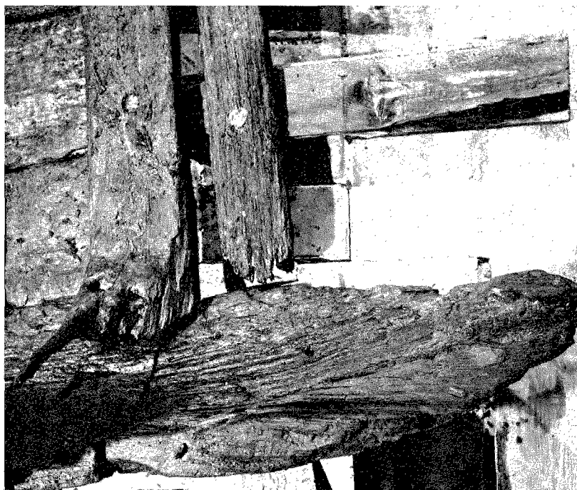
2 Druten: idem, curved end of transition strake, seen from above
