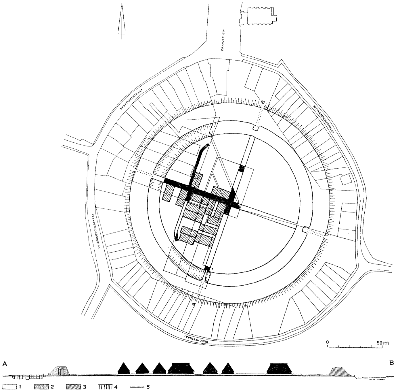
Fig. 4 Schematic plan of the Oost-Souburg fortress with moat, rampart, cross-roads, and the oldest house-sites; 1: raised layer; 2: view of the rampart; 3: section of the rampart; 4: stakes; 5: old surface
