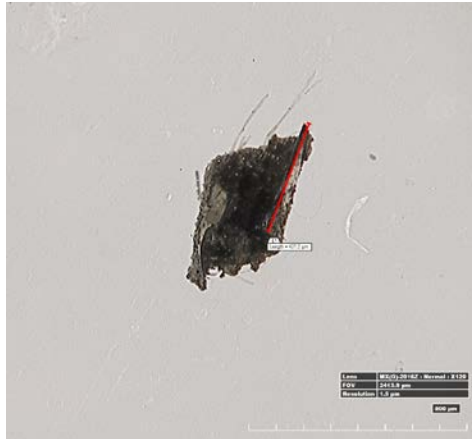
Figure 5.2. Sample 2: flat metal strip measuring 421.2 \mu\text{m} in width. X120, Hirox.
