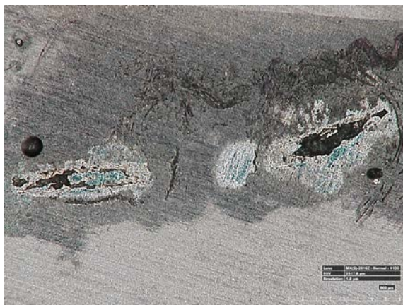
Figure 5.8. Sample S9 : spangle. Hirox, X160.
