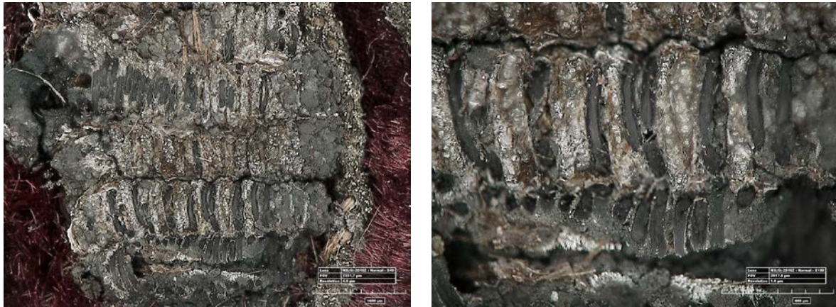
Figure 7.9-7.10. Hirox images of splitting round wire.
