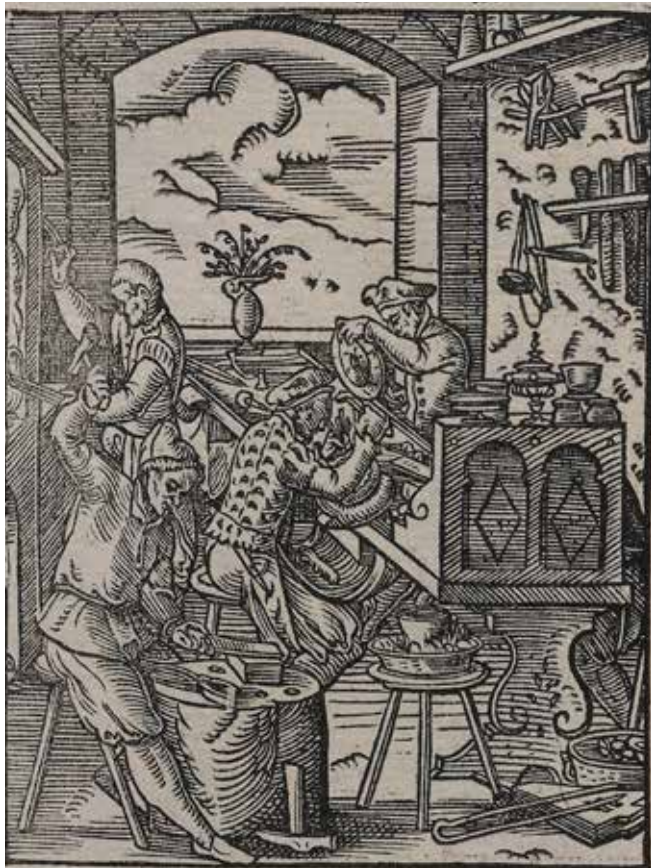
Figure 13 The interior of a goldsmith's workshop showing various products and tools, and men embossing and chasing metal vessels, beating a strip of metal and working at the fire. 'Aurifaber. Der Goltschmit (The Goldsmith)' from Panoplia omnium illiberalium mechanicarum ( Book of Trades ), 1568, woodcut engraving made by Jost Amman, published in Frankfurt by Sigmund Feierabend. British Museum, 1904.0206.103.16
