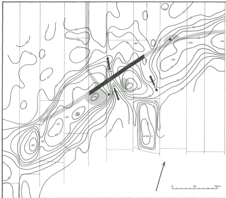
Fig. 28. Contour map of a part of the Schoonrewoerd stream ridge with the double break-through channel at "Ottoland-Kromme Elleboog". Indicated are the sites nos. 36 and 37. Excavated part of road under construction in black. Legend : see fig. 27. Scale 1:4000.
